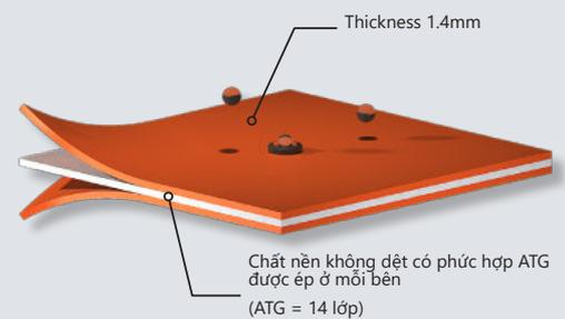
The ML31 complex is made up of two ATG barrier films laminated onto a non-woven substrate.
