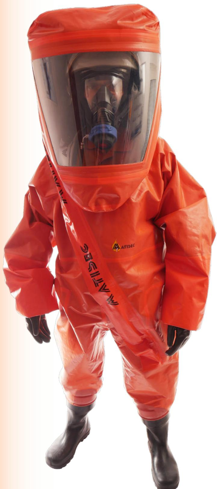
The DM II is a reusable protective suit that protects the user from chemical products in liquid or gaseous form, including liquid aerosols and solid particles. It is a non-ventilated, type 1a-ET suit (gas-tight in conformity with standard EN 943-2).
